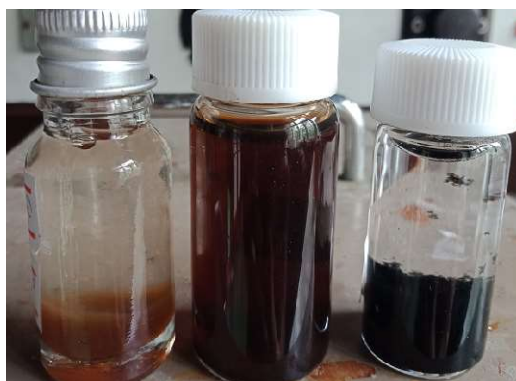
Figure 2 (a) Graphite oxide (b) Graphene oxide(GO) (c) Reduced Graphene oxide(rGO)
